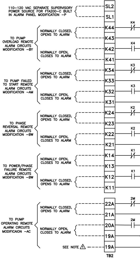
$\Delta$  SPARE TERMINALS PROVIDED FOR PARALLEL CONNECTION OF REMOTE ALARMS (IF REQUIRED)
